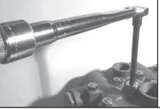
11. Place valve vasing (43) over studs and push firmly until seated against the crankcase (1). Tighten the hexagon nuts (49A) in a crosswise pattern (shown above) to 59 ft.lbs. (80 Nm).
