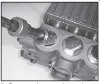
2. Remove the complete valve assembly (46) with valve pullers.
