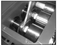
Separate plunger (36) from crosshead (25) by means of an open-end wrench (27mm).
