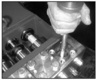
2. Remove tension spring (57) and complete valve assemblies (51 and 52) using either tool (part #07662) or stud bolt.
