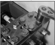
1. Loosen screws (58C), press plugs (58) out of valve casing with two screws - using them like "jack screws".
