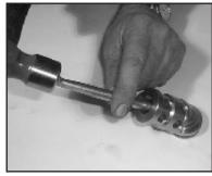
Valve seats (51C and 52C) are pressed out of spacer pipe (51F) by hitting the valve plate (51D) with a bolt.
