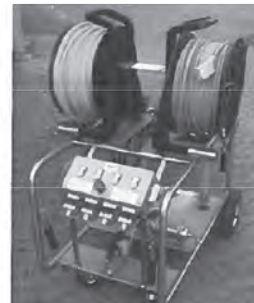
Design Example (left): Portable pneumatic control unit for up to four (4) operators. With four (4) valves, control box, cable reel and pneumatic hose reel.
