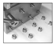
8) Loosen nuts (49A) with a 24mm socket wrench.
