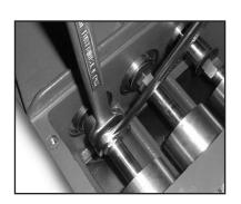
11) By gripping hex flats, separate plunger (36) from crosshead (25) by means of two open-end wrenches (size 22mm and 27mm).
