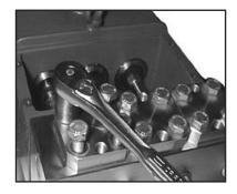
Loosen and remove screws (58C) with a 24mm socket wrench.
