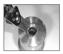
14) Remove circlip ring (48) from seal sleeve (38). Remove spacer disc (47) and seal ring (46) from seal sleeve. Replace worn or damaged parts.
