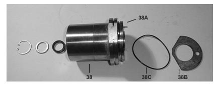
15) Remove leakage gasket (38B) from serrated pin (38A) on the seal sleave (38). Check o-ring (38C) for damage and replace if necessary. **IMPORTANT!** The 3.2 mm (diameter bore of the leakage gasket (38B) must be inserted directly on the serated pin (38A) of the seal sleeve (38). The leakage gasket must fit snugly to the seal so that the bevelled surface of the gasket faces outwords.
