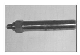
17) Examine plunger (36) for signs of wear or cavitation. If the surface of the plunger is worn, screw out the plunger with a 27mm tool. Clean centering and front surface of crosshead with plunger (25). Thread new plunger carefully through oiled seals in seal sleave. Coat thread of new plunger lightly with bonding agent (e.g., loctite).
