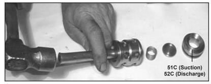
5) Valve seats (51C and 52C) are pressed out of spacer pipes (51F and 52F) by hitting the valve plates (51D and 52D) with a socket extention.
