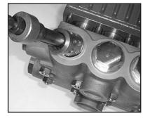
Remove the complete valve assembly (46A-46D) with valve pullers.
