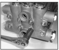
5. Loosen the 8 nuts (49A) with a 19mm wrench. Tap the back of the manifold (43) with a rubber mallet to dislodge and slide off the studs (49).
